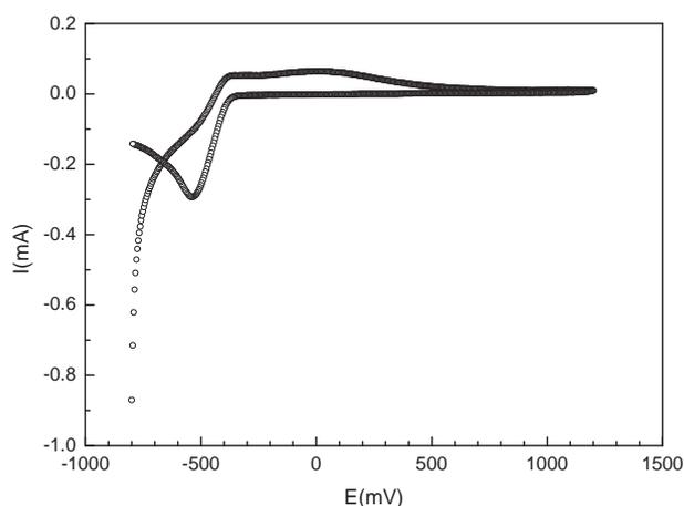
**Fig. 6. CV at pH=1.86 for the solution of 34.16x10<sup>-2</sup>% E<sub>4</sub> in 0.1M NaClO<sub>4</sub> at a scan speed of 50 mV/s**
