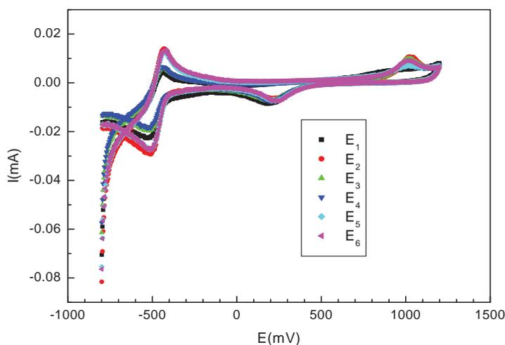
**Fig. 3. CV of the 6 types of Enoxil at  $4.95 \times 10^{-2}\%$  in 0.1 M  $NaClO_4$  at a scan speed of 50 mV/s**
