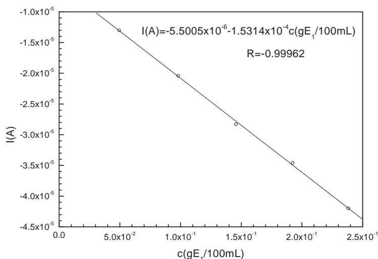
**Fig. 2. Dependence of the cathodic current intensity on Enoxil concentration ( $E_1$ ) in alcohol solution of ITBA**
